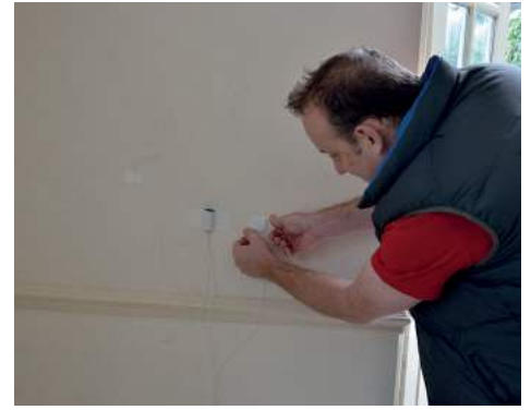
Pre-treatment set-up of U-value testing sensor
