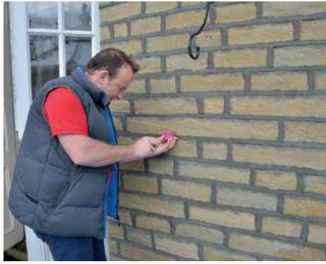
Exterior set-up of U-value testing sensor
